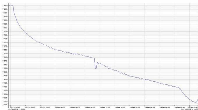
The graph shows the dramatic 80cm drop in flood water levels achieved in two days in February 2014 by fully opening the sluice at Monk's Leaze Clyse at the head of the Sowy (pictured right, branching off from the Parrett).
